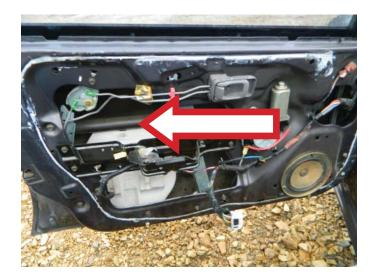
**STEP 9:** Once the window glass has been disconnected from the window regulator, manually slide the window glass into the closed position and hold in place with either a saddle cup assembly, painters tape, or a wedge.
