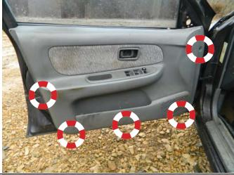
**STEP 1a:** Remove the door cup handle retaining screw.
