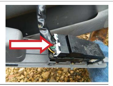
**STEP 4:** Using either a trim panel removal tool or small flat-blade screwdriver, remove the interior door handle bezel assembly.
