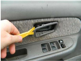
**STEP 2:** Using a trim panel removal tool, place the tool between the door and the interior door trim panel and using firm, even pressure release the interior door trim panel from the door.
