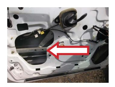
**STEP 2:** Using a 10 mm socket and ratchet, attach the window regulator rail to the door.
