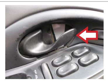
**STEP 12:** Verify that all of the interior door trim panel retaining screws are tight and the window regulator is operating properly.
