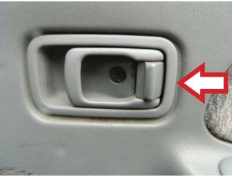
**STEP 5:** Using a trim panel removal tool, place the tool between the door and the interior door trim panel and using firm, even pressure release the interior door trim panel from the door.
