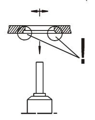
When fitting the spring plate ( 1 ) care must be taken to ensure that the circlip ring ( 2 ) is seated correctly!
