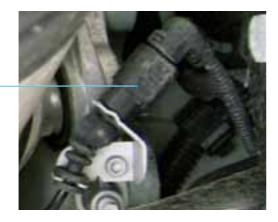
Loosen screw connection on spring strut 4
