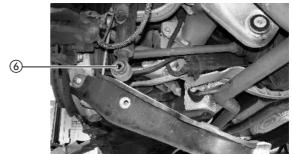
■ Push the bottom track control arm down and remove the strut sideways.
