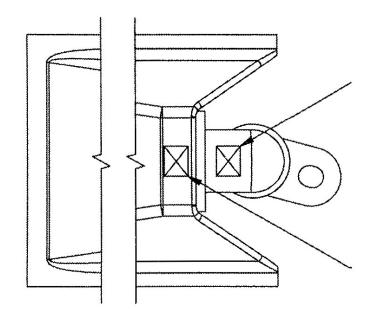
Apply pressure at this location to assemble strainer to pump.
